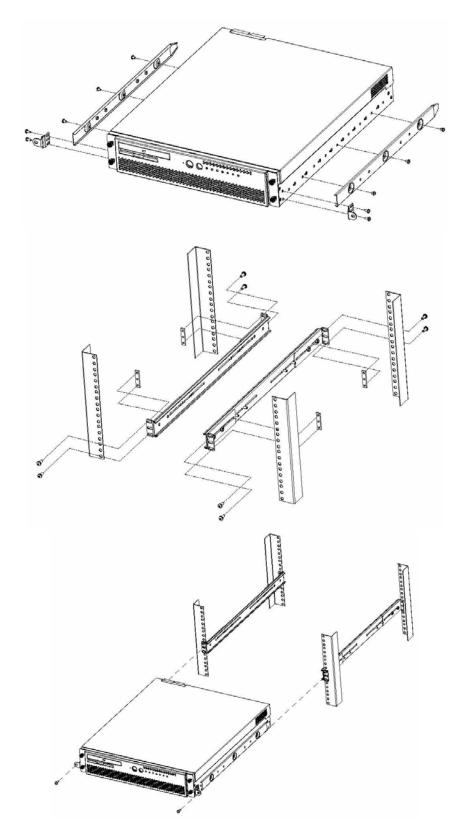
The diagrams above summarize the components and "slide-in rail-type" system of the TMLPMOUNT41. It can be adapted for a 2-post or 4-post installation.
